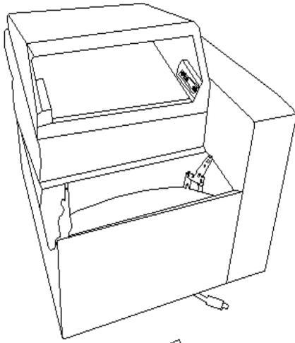
Be cautious when routing the cables. The cord can be damaged by the mechanism if routed too close during installation.
