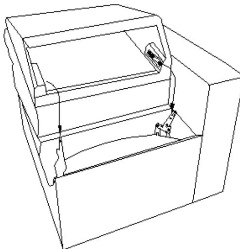
Lay Seatback face down on seat. Align the mechanism tongues into the backrest slot while lifting the backrest into the upright position. Slide the seatback onto the tongues while pressing downward until both sides engage. You will hear a click sound from each side. Firmly pull up on the backrest to ensure engagement of both attachment points.
